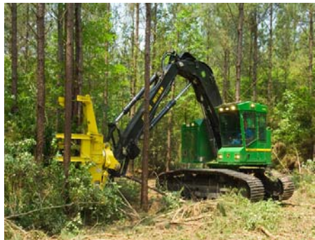
FIGURE 2: MECHANIZED EQUIPMENT USED TO FELL, SKID 8 , CHIP AND TRANSPORT P-J BIOMASS
